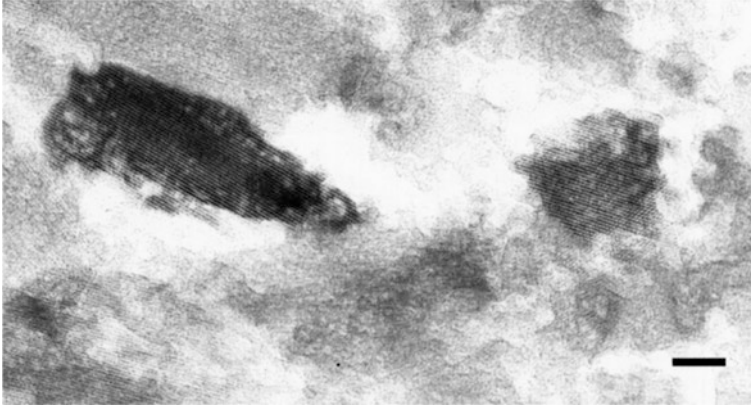
Fig. 2.8 TEM observations of calcium phosphate mineral in the core region. Two apatite crystals are confirmed. No stain. Bar = 10 nm
