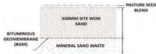
Figure 2. Schematic of mineral sand waste capping solution.
