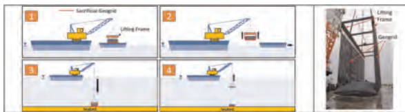
Figure 2. Installation using high-capacity crane barge (left) and lifting frame with geogrid setup (right).
