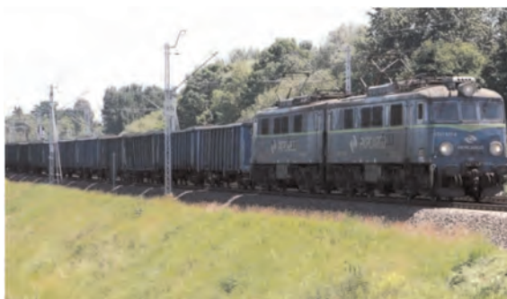
Figure 3. Live load example – LM71.
