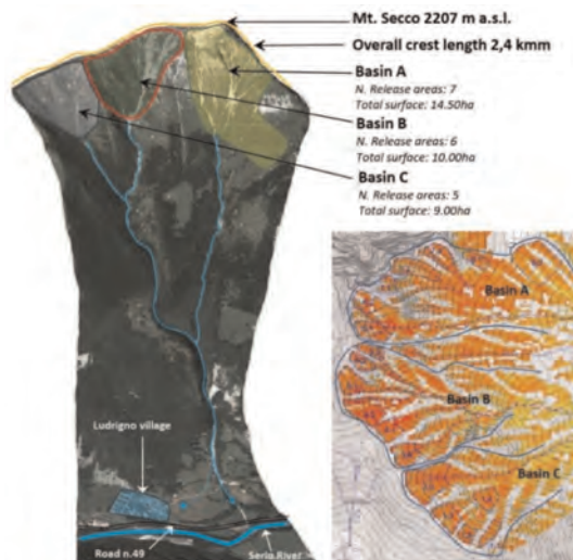
Figure 1. Main avalanche features (left) and PRA outline (right).
