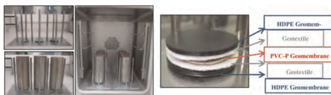
Figure 6. Plasticizer migration test. Arrangement of the test pieces in the combination that includes a separator geotextile, for carrying out the plasticizer migration test.
