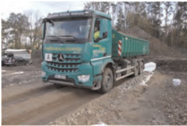
Figure 4. Ruts of a fully loaded truck.
