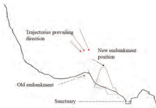
Figure 2. Effect of embankment relocation.
