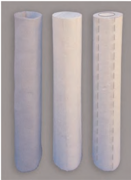
Figure 1. Reinforcement materials: (a) Hollow Geofoam, (b) Normal Geofoam, (c) Geotextile.
