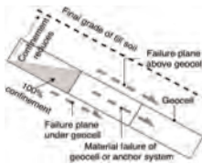
Figure 1a. Modes of failure.
