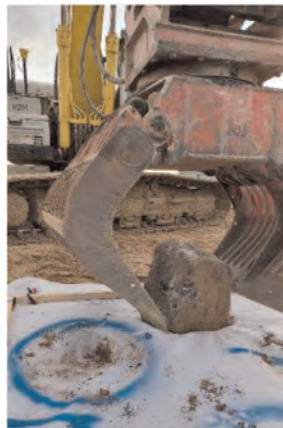
Figure 9. Fieldtrial drop tests with selected stone classes on nonwoven geotextile and analysis of failure mechanism and test conditions subsoil.
