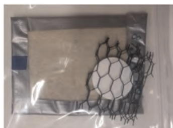
Figure 1. Filter paper setup for measuring total suction.
