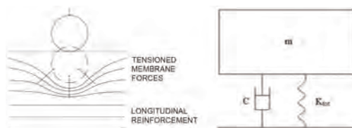
Figure 2. a) Elastic resistance of the longitudinal reinforcements through the tensioned-membrane effect; b) Scheme of the 1-DOF oscillator.
