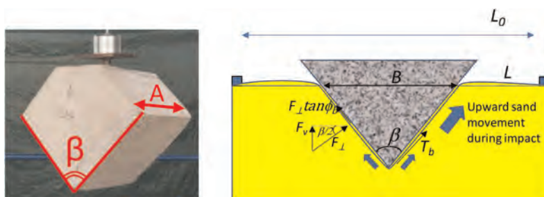
Figure 3. Block type used in model and definition sketch. L is the length of the elongated geotextile. The arrows indicate the sand movement along the geotextile.
