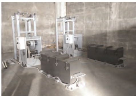
Figure 1. Large-scale prototype apparatus for long-term pullout tests.
