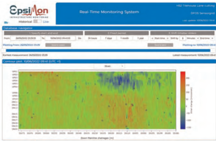
Figure 17. Visualization dashboard displaying strains in monitored section at Tilehouse lane cutting.
