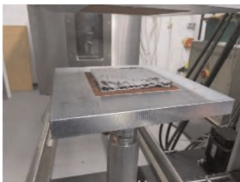
Figure 6. Compression test specimen before realisation of test in temperature-controlled chamber. The temperature-controlled chamber can be seen at the back of the photo.
