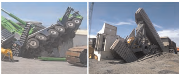
Figure 1. Examples of construction machinery overturning.
