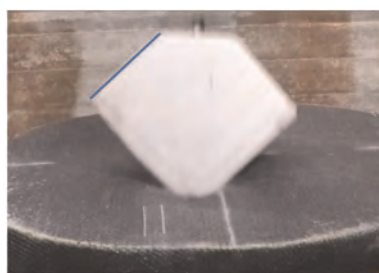
Figure 6. Maximum penetration of block taken from high-speed video (250 fps), see also text.
