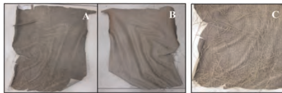
Figure 4. PVC-P geomembrane sample extracted from the north slope crest 258 months after re-waterproofing. A: external face, in contact with the HDPE geomembrane, B: internal face, in contact with the geotextile, C: detail of the state of the external face of the geomembrane.
