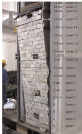
Figure 5. Displaced wall facing after application of extreme acceleration.
