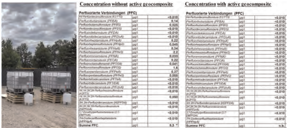
Figure 20. Outdoor trials with active geocomposite for PFAS and results of Rain Event 3, (Huesker Ltd.).
