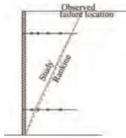
Figure 2. Estimated failure plane based on reinforcement strains and top topography.
