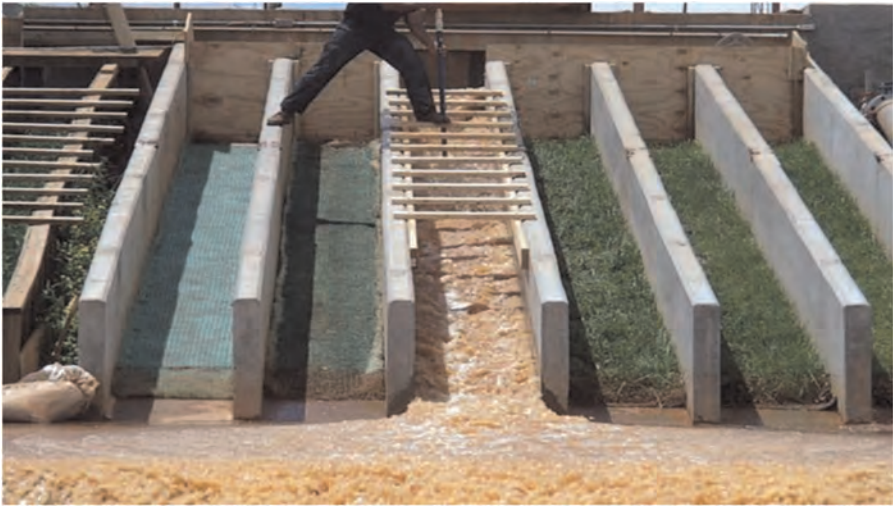
Figure 11. Large-scale channel erosion testing facility.
