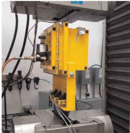
Figure 4. Composite stiffness test apparatus (courtesy of TRI Environmental, Inc.).
