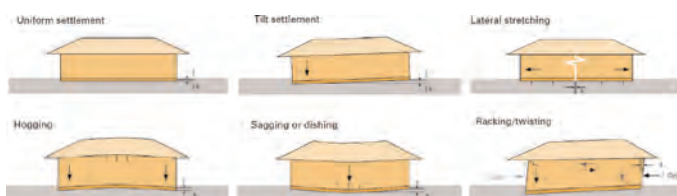
Figure 1. Typical damage patterns for house foundations, after (Department of Building and Housing 2011).
