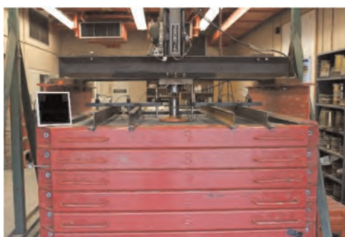
Figure 1. Example of large-scale laboratory box test setup.
