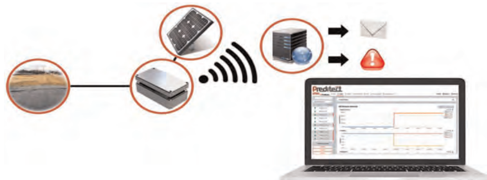
Figure 4. Operating principle of the measurement chain and monitoring of the integrated survey system.
