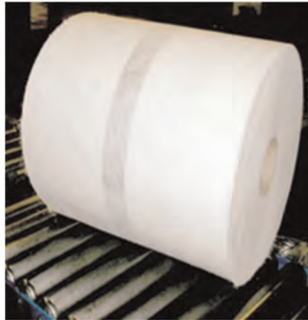
Figure 10. Non-woven polypropylene incorporating a 50 mm wide aluminium foil (Terram Ltd).
