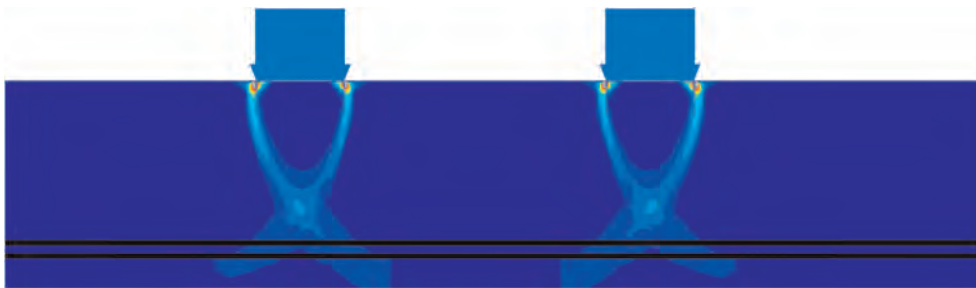
Figure 5. Failure within a thicker working platform with insufficient shear strength ( h_{\text{platform}}=2\text{ m} , \varphi_p=27^\circ ).
