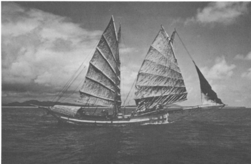
Plate 6. The perahu pinas dogor under sail makes use of dipping lug sails, made of mengkuang reed matting, stiffened with battens.
