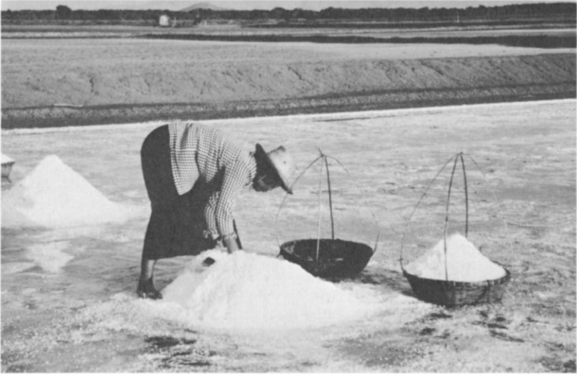
Plate 1. Salt is manufactured by the evaporation of sea water on coastal salt fields close to the small port of Ban Laem, Thailand.
