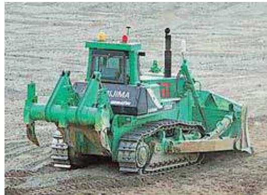
Fig. 3. Multiple cooperating construction robots are operated by a single human supervisor from a central box, Vision Sketch Japanese Research Institute, 1980
