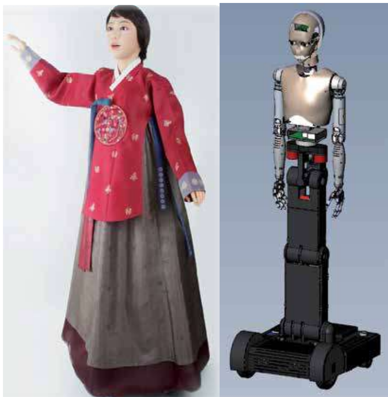
Fig. 1. The android robot EveR 3 and its mechanical drawing.
