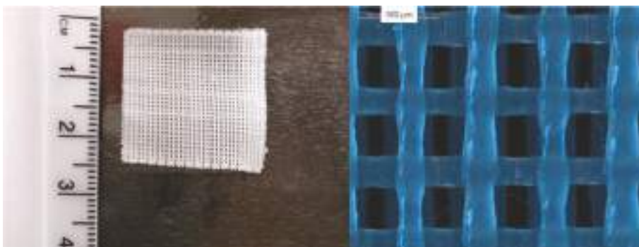
Figure 2. Macroscopic (left) and light microscopy image (right) of the 3D printed film.
