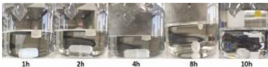
Figure 5. Photographs of 3DP tablet (T2) floating in dissolution medium (0.1 N HCl solution) at room temperature.
