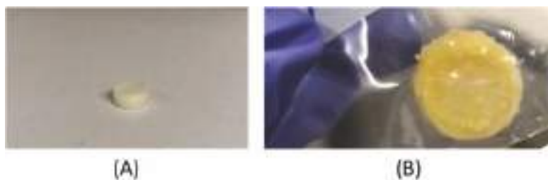
Figure 4. Representative image (A) printed PVA product and (B) three-dimensional (3D)-printed fixed-dose combination (FDC) drug product with dimensions 10.45 \times 10.54 \times 3.79 mm.
