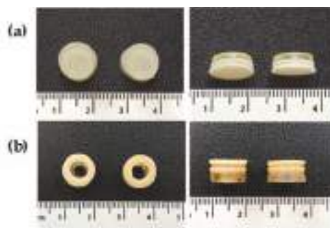
Figure 2. Polypill printlet (a) Type I (cylinder shape) and (b) Type II (ring shape). The Type III formulation was visually identical to Type II, and hence, has not been included here. The scale is in cm.
