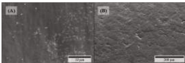
Figure 3. SEM pictures of filaments without any API: (A) HPMC surface; (B) PEO surface.
