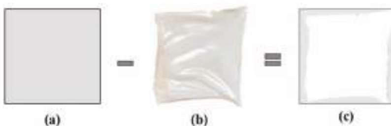
Figure 1. Theoretical dimensions of the patches (a), experimental dimensions of the 3D-printed patches after drying (b), and their difference (c), as it is calculated by Equation (1).
