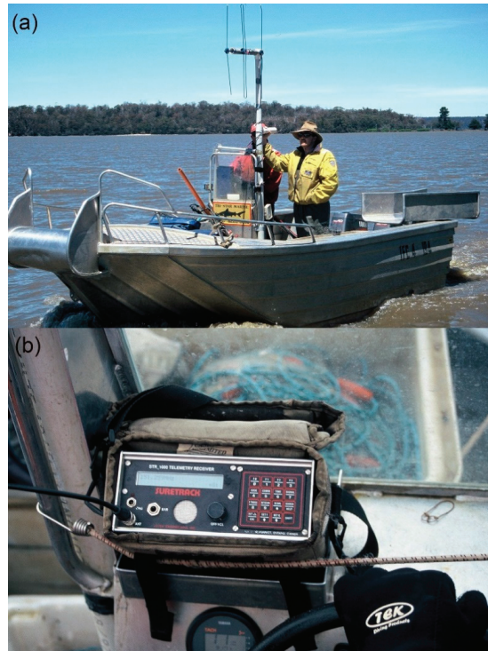
Figure 3. A CMP work boat with a directional antenna installed (a), hooked up to a Lotek telemetry receiver (b) for tracking and monitoring transmitter carp.
