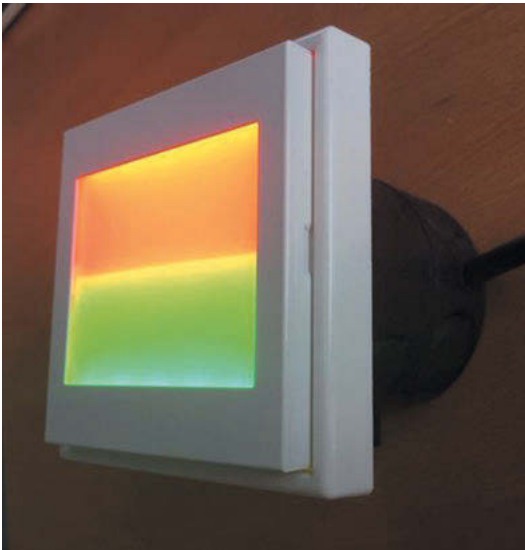
Figure 4.3: Prototype of an energy signal light to be build flush-mounted.
