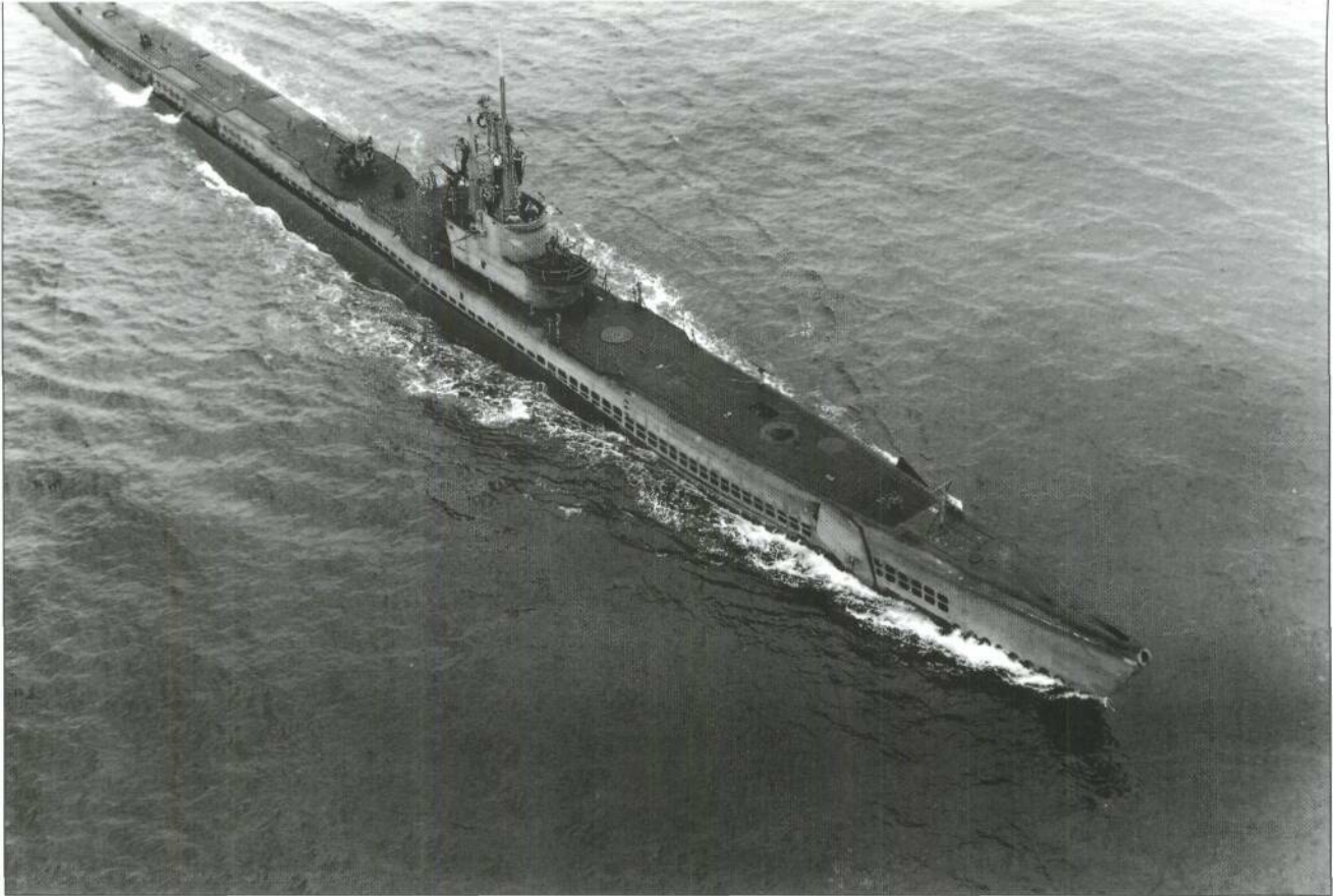
Above: USS Argonaut , second of the name, in April 1945. The forward deck gun has given way to a short 5in gun abaft the conning tower, a 40mm Bofors and twin 20mm guns aft.
