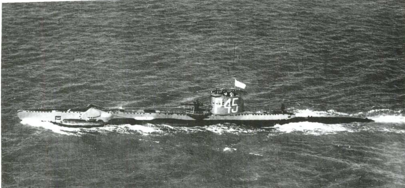
Above: HMS Unrivalled , one of the improved 'IT class. They could be distinguished from the pre-war boats by their 'shark' bow. Designed for training, they also saw combat.
