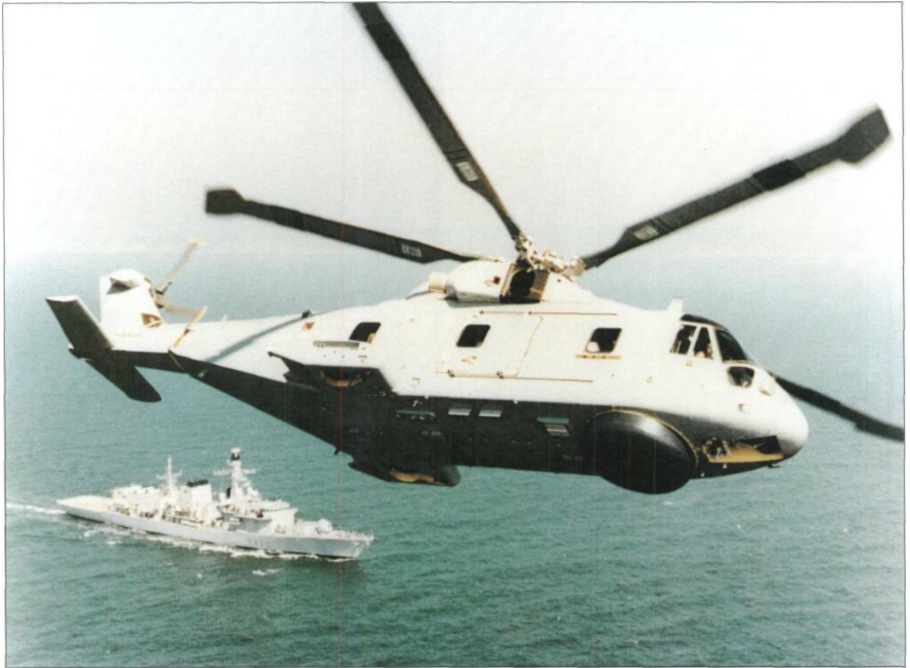
Above: The Augusta-Westland EH101 Merlin is the Royal Navy's new anti-submarine helicopter (due 1999). Its three gas turbines provide range and a large safety margin.
