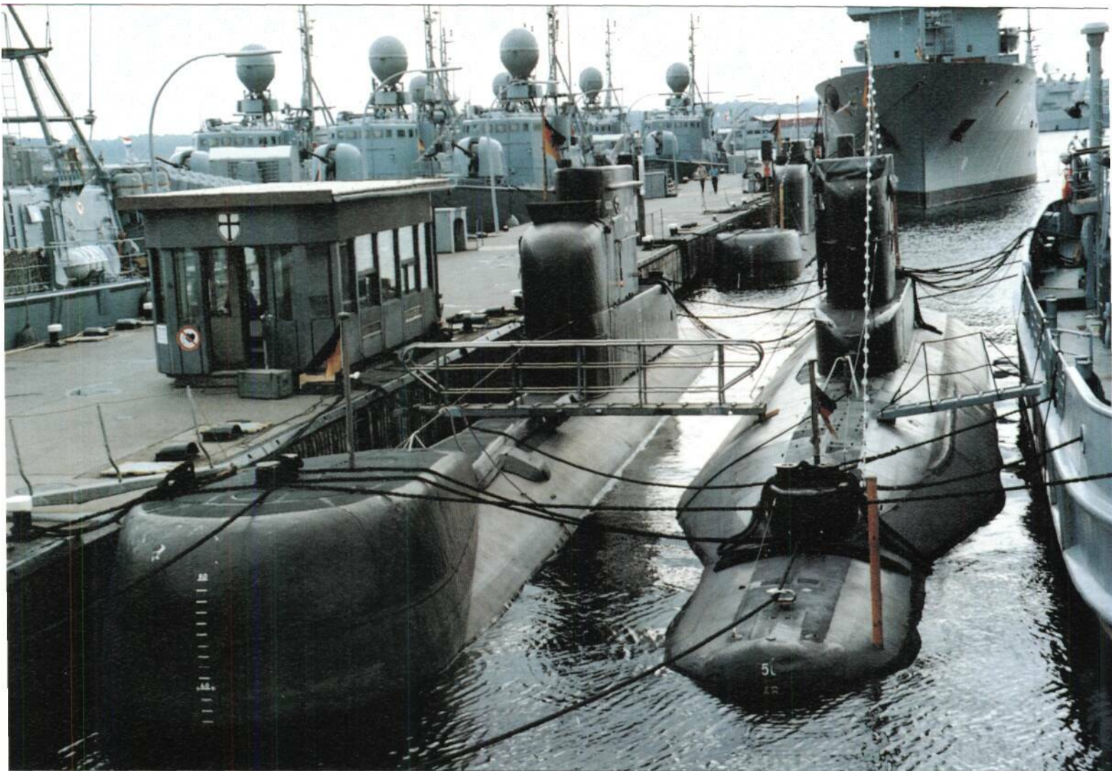
Above: Two Type 206A submarines at Kiel in 1995. Some 18 were built in 1971-74 and armed with DM2A1 Seeschlange wire-guided torpedoes, plus DBQS-21D sonar in the bow.
