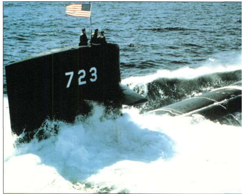
Above: The streamlined fin of the USS Oklahoma City . The 'Los Angeles' design emphasised high pursuit speed by doubling the output of the S6G reactor.
