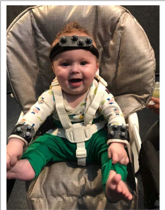
FIGURE 2 | Motion tracking systems allow for precise tracking of infant's limb or head movement. The position of light reflecting spheres attached to the infant body is triangulated with the help of a system of surrounding cameras. This system is light and does not interfere with infant's movements.
