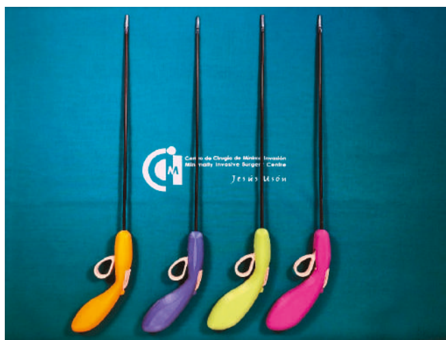
Figure 2. Prototypes of the handles for laparoscopic instruments developed. The sizes of the handles, from left to right, are XS, S, M and L.
