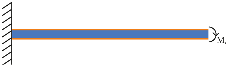
Figure 3. Piezoelectric action (PIN force model).
