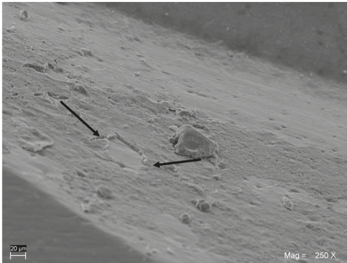
Figure 4. Group 1. Aspects of the steel drill after 50 disinfection cycles with glutaraldehyde, where zones of structural alteration can be observed.
