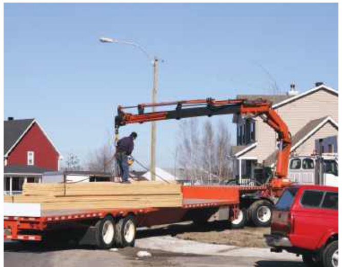
Figure 9-6. Truck-mounted crane. Source: http://www2.worksafebc.com/PDFs/construction/types_of_cranes.pdf and http://overtonsafetystore.com/images/Sheetrock%20Boom%20Truck.jpg .
