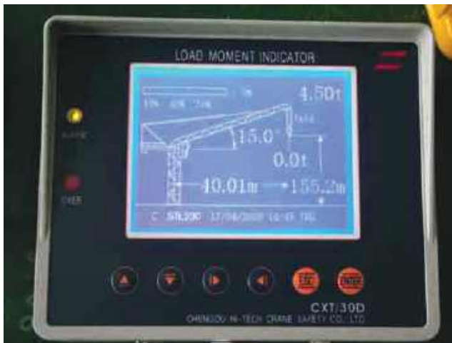
Figure 9-17. Hardware used to measure and display the real-time load moment on crane during operation. Source: Cranesmart.
