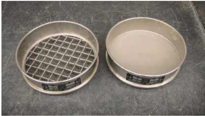
Figure 6-1. Sieves with 19.0-mm and 0.075-mm openings. A stack of many sieves having progressively smaller openings from the top sieve to the bottom becomes the “nest” or array of sieves through which the sampled soil is shaken in order to obtain data by which to begin the soil classification process.
