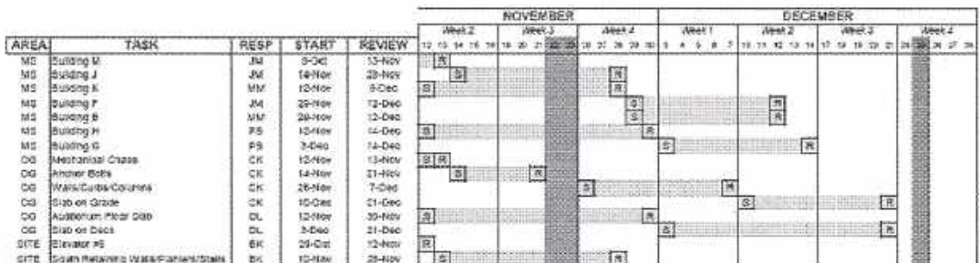
Figure 5-14. The schedule keys the lift drawing to the period when the work will be done.
