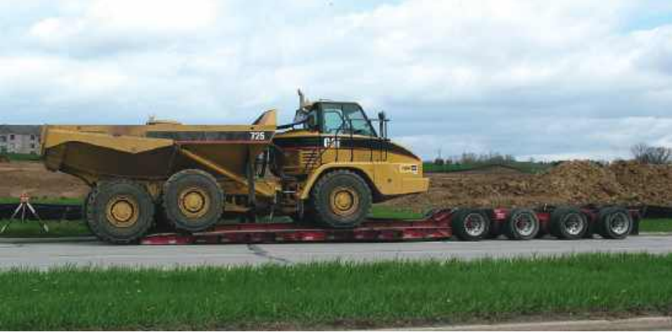
Figure 8-6. Off-road articulating truck loaded onto a “low-boy” trailer for street travel.
