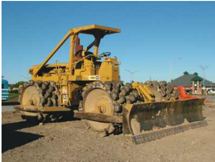
Figure 6-20. Self-propelled sheepfoot roller. A sheepfoot roller is usually applied for fine-grained soils. A suitable weight and type of roller applied to fine-grained soil near the OMC usually compacts the fill to the specified percentage of \gamma_{d,max} within six coverages. When a sheepfoot roller “walks out” of the soil (i.e., when the compacted soil supports the roller without allowing the feet to penetrate the surface), it has reached the limit of its effectiveness for the conditions. The blade levels the surface of the loose fill so that the compaction effort is more evenly distributed.
