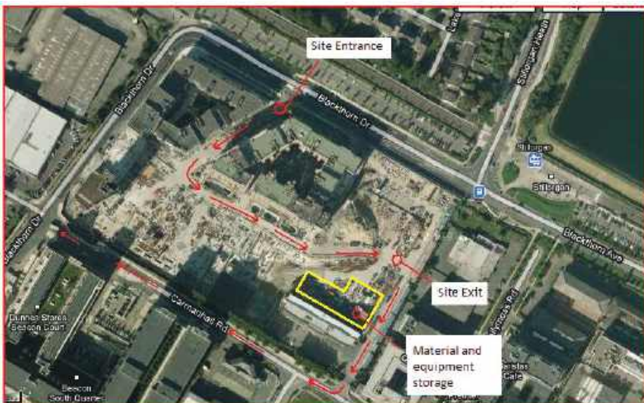
Figure 4-35. Site entrance, temporary roads, and material storage locations.
