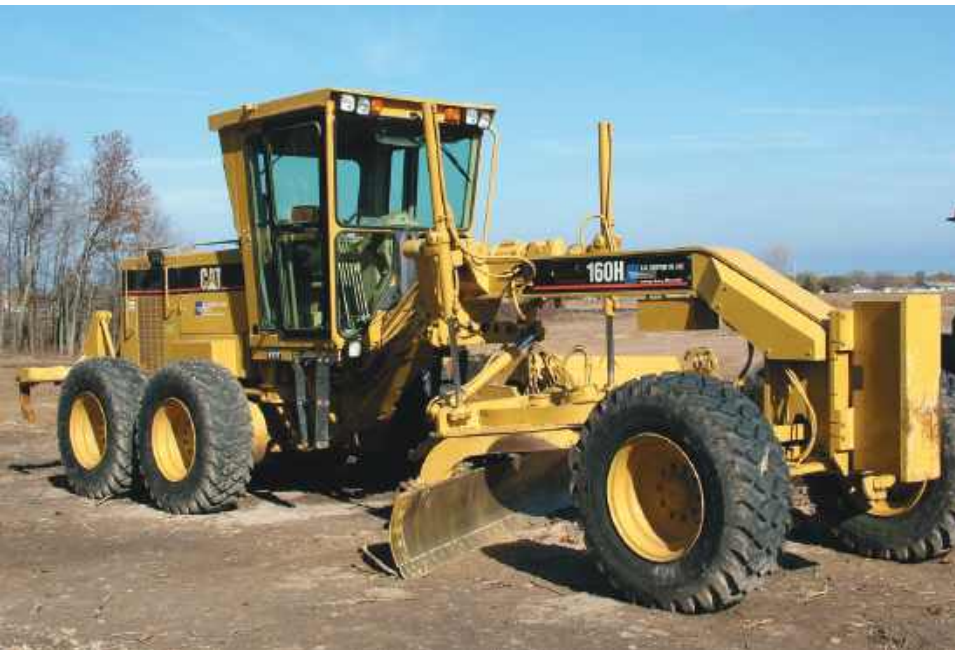
Figure 8-7. Motor grader. Note the light-duty ripper-scarifier mounted on the back end.
