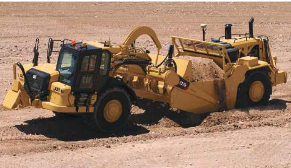
Figure 8-5. A 21-cy capacity elevating self-propelled scraper.
