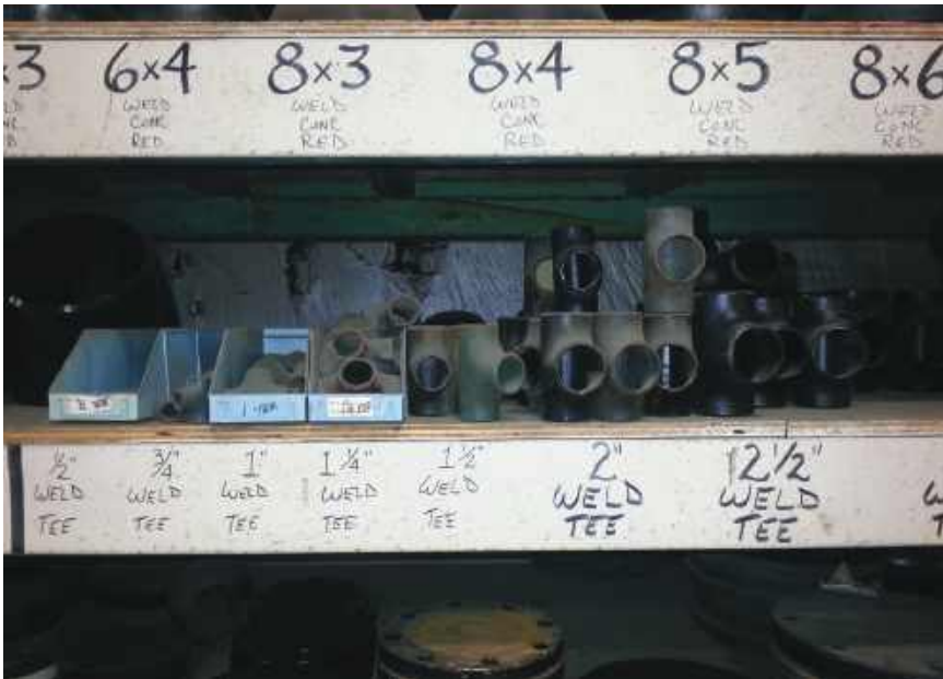
Figure 7-15. Exact and open locations for materials to avoid searching and assist in reordering.
