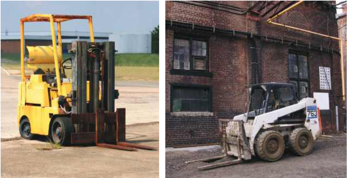
Figure 9-9. Standard fork truck (left). Skid steer loader with forklift attachment (right) Source: www.photos.com .
