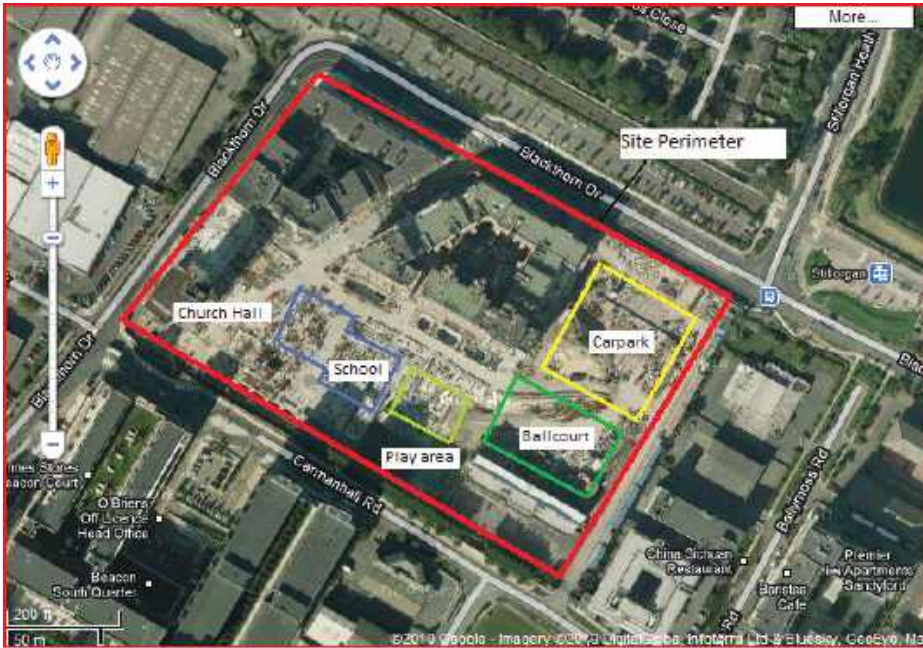
Figure 4-34. Overlay of the buildings on the site. This was done using a scaled version of the building put in the relevant locations on the site. Note that some of the parking, ball court, and play areas have changed locations with the agreement of the architect and the client.
