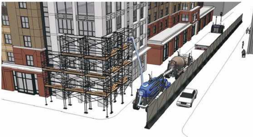
Figure 7-4. Sample BIM to show logistics plan.
