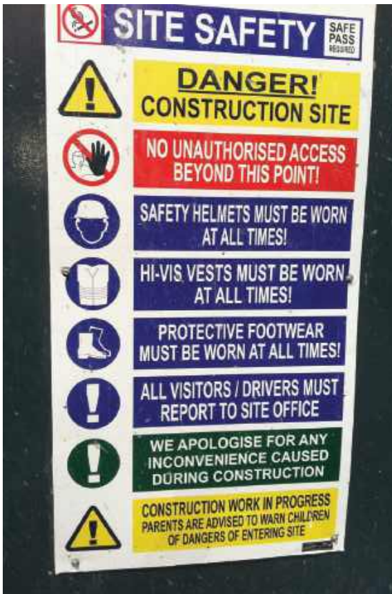
Figure 4-8. Typical site safety signage used during construction.
