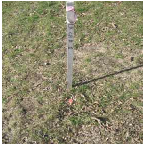
Figure 5-4. Contractor primary control.
