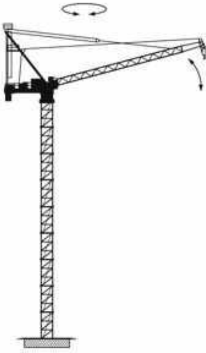
Figure 9-8. Tower crane with luffing jib. Source: http://www2.worksafebc.com/PDFs/construction/types_of_cranes.pdf and www.photos.com .
