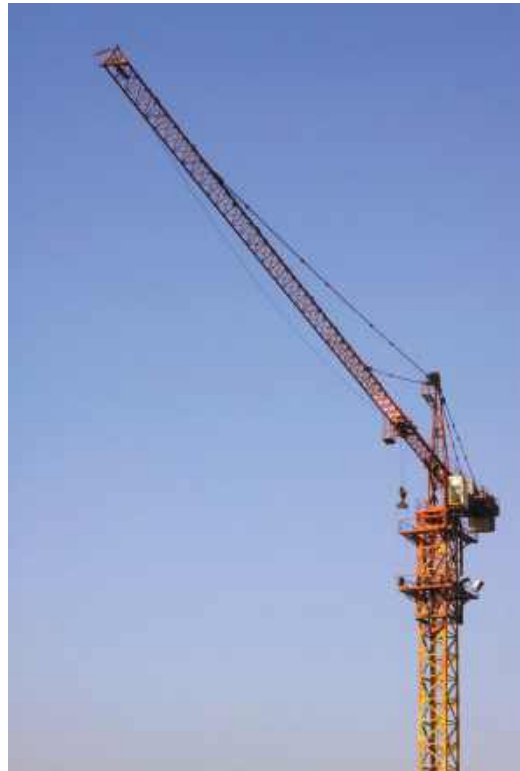
Figure 9-8. Tower crane with luffing jib. Source: http://www2.worksafebc.com/PDFs/construction/types_of_cranes.pdf and www.photos.com .
