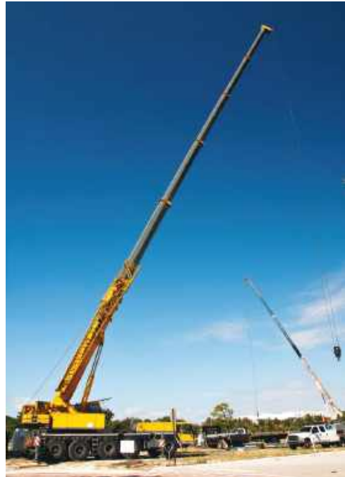
Figure 9-5. Wheel-mounted mobile crane with telescopic boom. Source: http://www2.worksafebc.com/PDFs/construction/types_of_cranes.pdf and www.photos.com .
