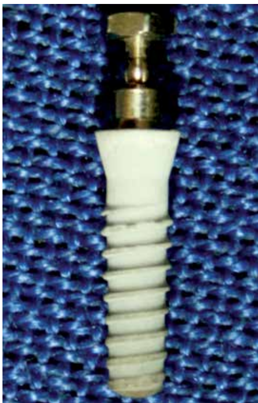
Figure 7. Hydroxyapatite-coated titanium implant.
