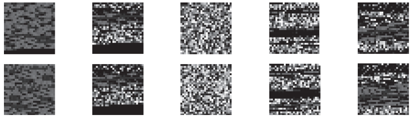
Figure 6. Traffic visualizations of trojan Zeus (the first column), Skype (the second column), Outlook (the third column), backdoor Htbot (fourth column) and botnet Virut (fifth column). Images were created by the authors with the advantage of the tool introduced in [34] on the USTC-TFC2016 dataset.
