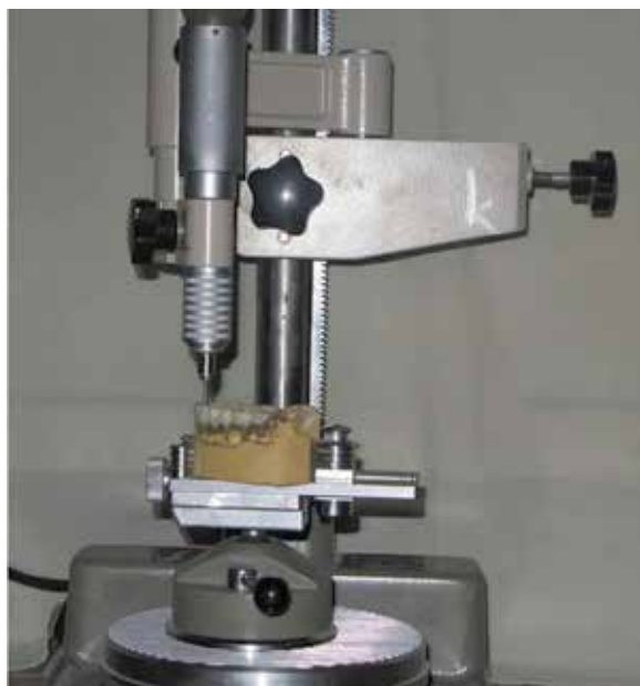
Fig. 1. A scheme of the preparation of implant access holes along the long axis of teeth using milling machine.
