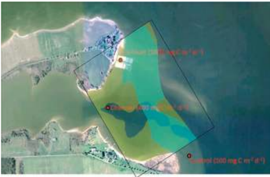
Fig. 24.7 Erosional area from tides (light green) and waves (dark green) with the sedimentation rates indicated on an oyster farm, channel and control areas in Maryland, U.S.A. (Testa et al. 2015)
