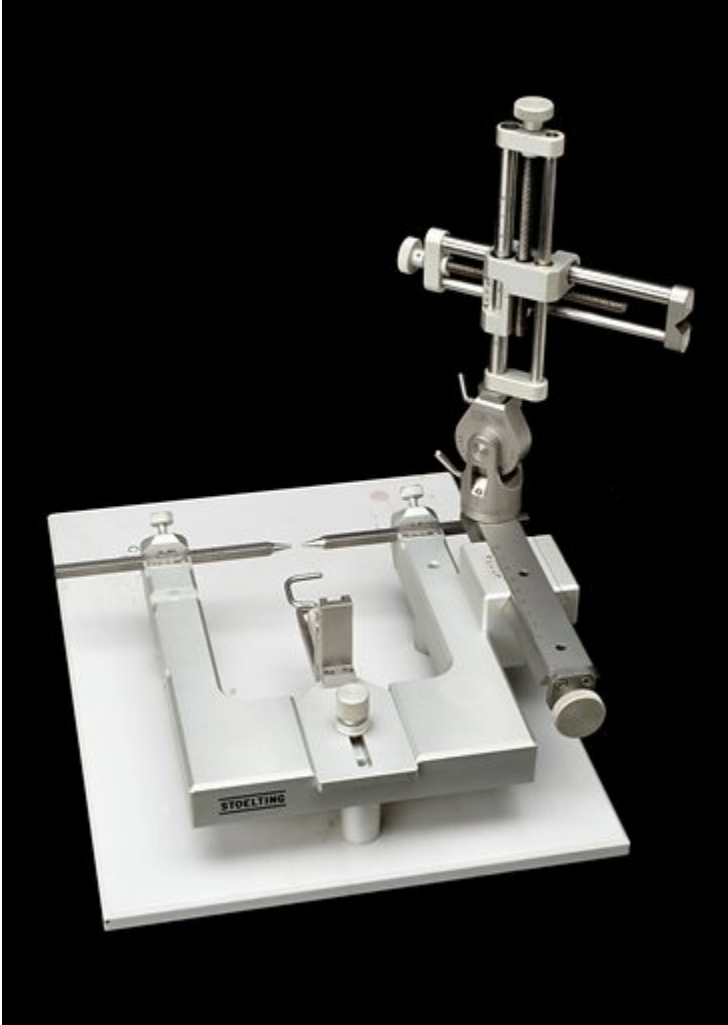
Figure 4. A stereotaxic device used to perform surgeries on rodents. This unit would immobilize an anesthetized rat and allow precise placement of electrodes in the brain.
