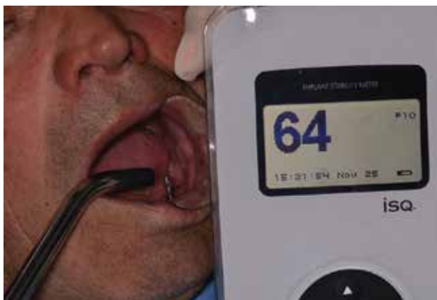
Figure 1. Resonance frequency analysis measurement using Ostell Mentor® device.
