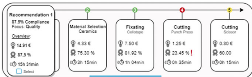
Fig. 5.9 Illustration of a recommended process configuration from the FRP process chain planning tool with a global evaluation of the whole chain on the left and local information on possible problems on the right
