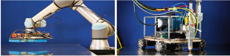
Fig. 20.1 MVP of a Tool Center Point sensing unit (left), MVP of a mobile robotic system for laser material processing (right)
