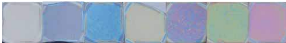
Figure 1. Photograph of a series of NH 2 -MIL-88B films deposited on silicon wafers with various concentrations (from left to right: 0.5, 1, 2, 3, 4, 5, and 6 wt%) by spin-coating method. Reproduced from Ref. [16] with permission from The Royal Society of Chemistry.
