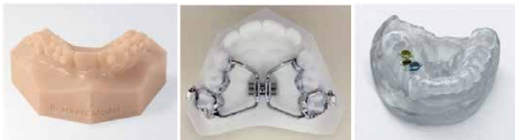
Figure 27. Dental model, RPE, and an implant surgical guide 3D printed from a STL generated file [38, 86]
