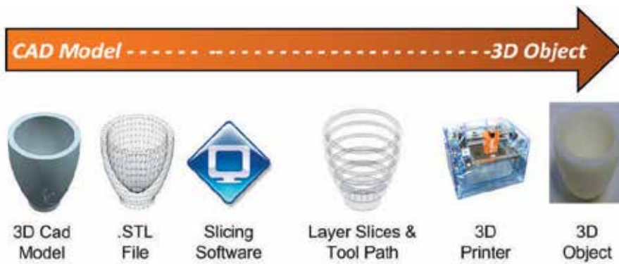
Figure 19. The 3D Printing process [79]
