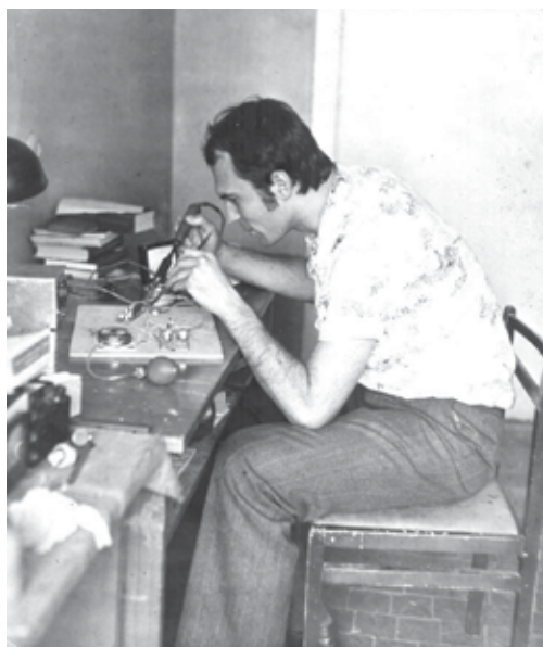
Fig. 7. M. Rudenko is in the hostel soldering the pressure-voltage transformation junction. The strain indicator is glued to the shoe cream box. Thus, the Big Science started (1978).
