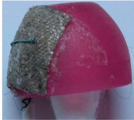
Figure 4. Single channel electrode used in the experiment using earphone rubber and silver-adhesive fabric electrode.
