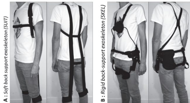
Figure 2. The two exoskeletons used; (A) soft back-support exoskeleton or exosuit (SUIT) (Corfor ® -V2, Villemus, France), and (B) rigid back-support exoskeleton (SKEL) (Laevo ® -V1, Deft, The Netherlands).
