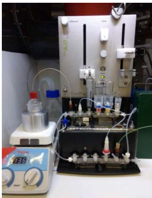
Figure 1. TRASIS mini AlliOne (miniAiO) setup for purification of zirconium-89.
