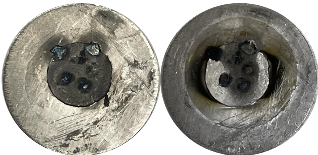
Figure 1. Representative image of a 7.9 mm \phi , 270 \mu m-thick, 106 mg holmium disc spot-welded to tantalum, before and after 68 min, 40 \mu A·h PETtrace irradiation.
