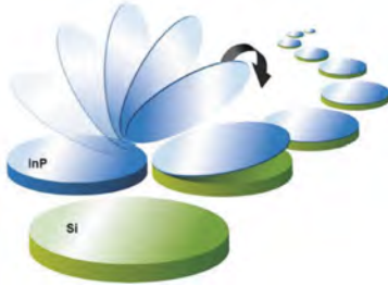
Fig. 3. InPoSi wafer fabrication principle (SOITEC SMARCUT™ process).
