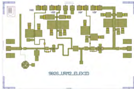
Fig. 3. PA layout. Chip size is 3.0 mm × 2.0 mm.
