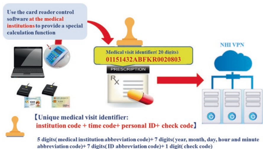
Fig. 10.10 The principle of the medical visit identifier production system and the providing method
