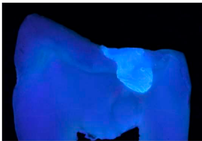
Figure 2. Image of a cross-section premolar slice in UV light (385 nm), revealing the differences in fluorescence between dental tissues and a restoration with Charisma ® . The digital equipment used was a DSLR camera (Nikon D3100) equipped with a macro objective (Tamron 90 mm), ISO 200, f/22, exposure time: 1/200 s.
