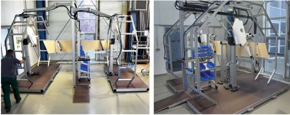
Fig. 4 The jig demonstrator with two mobile jigs and one stationary platform
