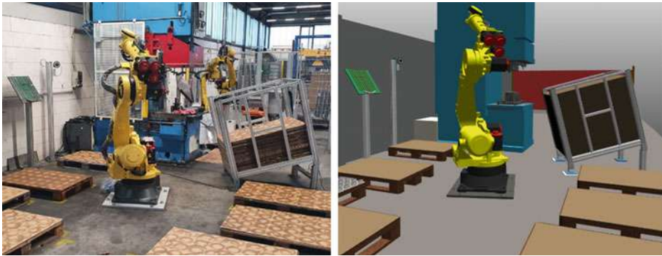
Fig. 3 Production process from aha! Albert Haag GmbH [1] and its digital twin
