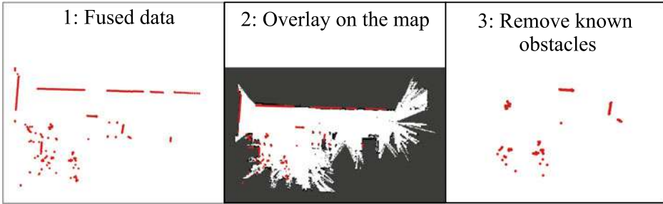
Fig. 3 Eliminating obstacles from the data based on the map
