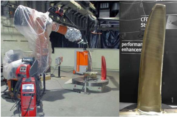
Fig. 6 Left: test setup for the build-up welding, right: welded demonstrator blade with mechanical finishing
