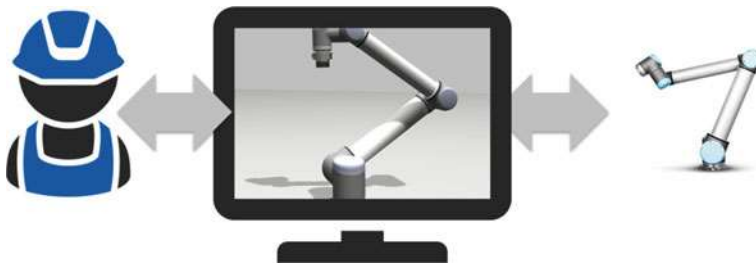
Fig. 3 Schematic concept of the digital twin as a mediator between the operator and the real twin
