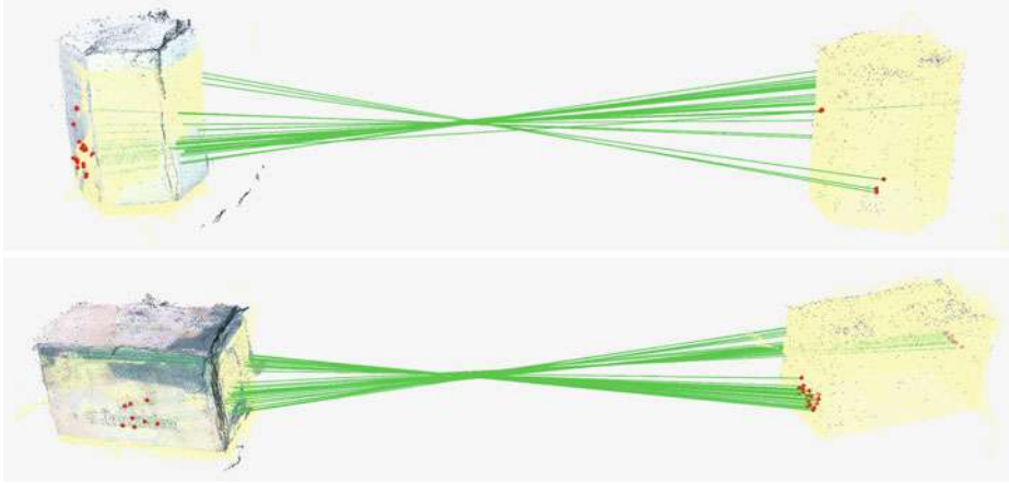
Fig. 4 Merging of two half-models of a pen box (top) and a tea box (bottom). One half-model is shown in original colours, while the other one as well as the resulting transformed half-model are shown in yellow. The keypoints are depicted in blue and correspondences as green lines, with their respective keypoints in red
