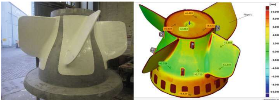
Fig. 5 Measurement results to illustrate the deviations of the casting surface from the planned one
