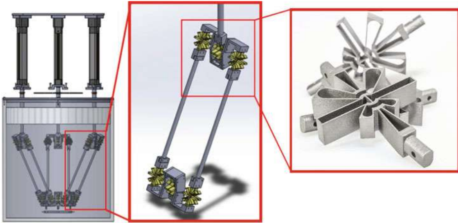
Abb. 2 Left: CAD rendering of a possible parallel robot structure (from [15]), middle: detail on the leg chain, right: flexure hinge photograph
