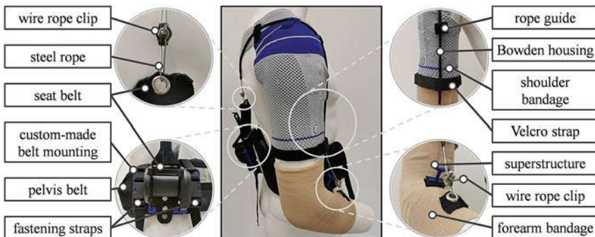
Fig. 3 Overview and central elements of the modular soft elbow support system
