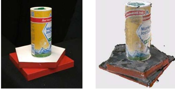
Fig. 2 An object with many symmetries and few edges and corners is placed on the calibration object (left). Multiple point clouds taken from different views can still be merged with the ICP algorithm due to the additional imposed edges and corners by the calibration object (right)
