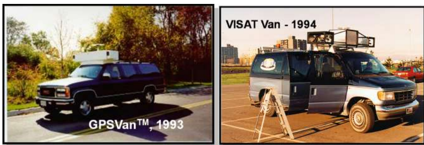
Fig. 25.4 The first land-based mobile mapping technology
