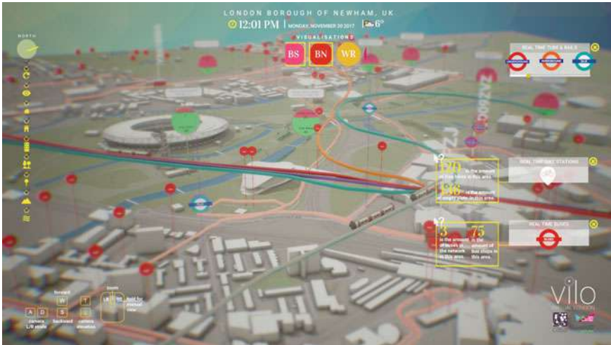
Fig. 38.2 QEOP in the “ViLO” model providing real-time IoT data within a 3D environment
