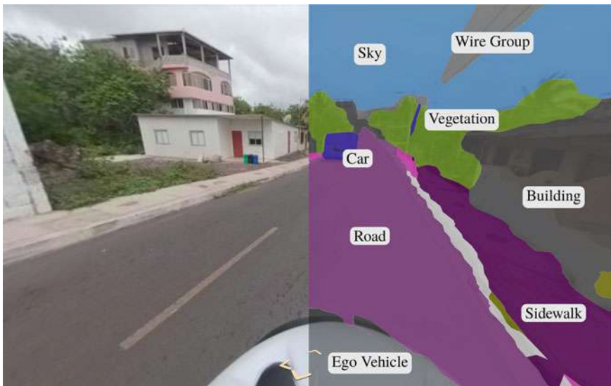
Fig. 4.2 Street-level imagery can be captured with relatively simple tools. For this study, we collected data by attaching a 360-degree sports camera on a helmet and rode a bicycle through the town. The imagery is available through Mapillary's (2019) user interface, as depicted on the left panel. The right panel shows processed and segmented imagery. The automatic object classification identifies structures and objects out of almost three-dozen categories. However, on the island, the algorithms sometimes fail to properly identify certain objects. For example, the sidewalk on the right is classified as ground. Nevertheless, the methods provide a powerful tool to assess urban features in developing towns experiencing rapid change
