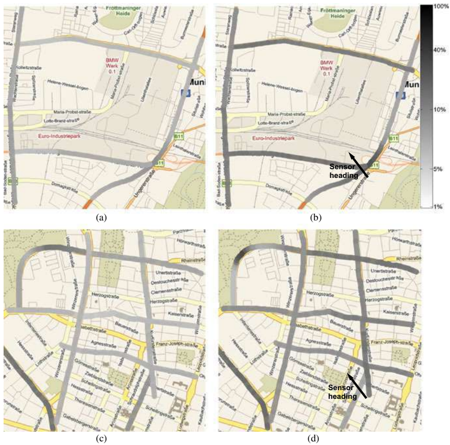
Fig. 22.11 Simulation of \sigma_v for two road networks north of Munich using the velocity estimation schemes: a The estimation accuracy for the first road network in % of the absolute velocity using the second scheme; b The estimation accuracy for the first road network in % of the absolute velocity using the first scheme; c The estimation accuracy for the second road network in % of the absolute velocity using the first scheme; d The estimation accuracy for the second road network in % of the absolute velocity using the second scheme
