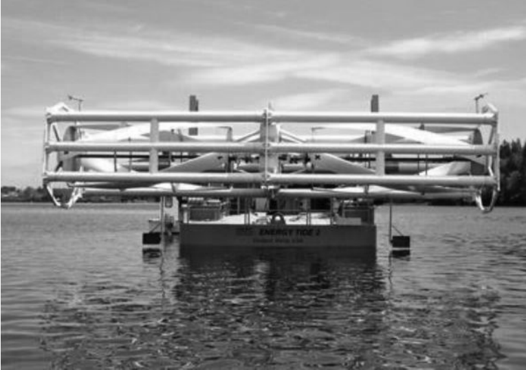
FIGURE 13.6 (See color insert.) Cross-flow turbine used in Alaska Rivers: ORPC's TidGen™ power system. [Adapted from “Hydrokinetic energy (in river, tidal, and ocean current),” Alaska Energy Wiki , Alaska Center for Energy and Power, 1–4, 2012.]
