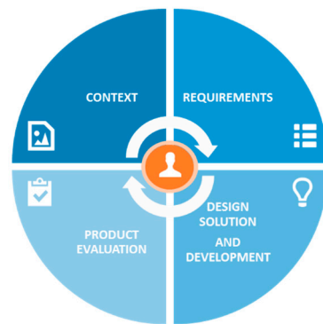
Figure 1. User-centered designed approach. Context: the program manager identifies who are the primary users of the product, how and why they will use it, what are their needs, and which environment they will use the tool. Requirements: when the context is defined, the program manager identifies the detailed requirements of the product, according to the needs of the user. Design solutions and development: once goals and requirements are settled, the ICT professionals and the project manager design and develop the tool for its usability. Evaluate Product: product designers (in this case, ICT professionals) run usability tests to obtain users’ feedback on the product.
