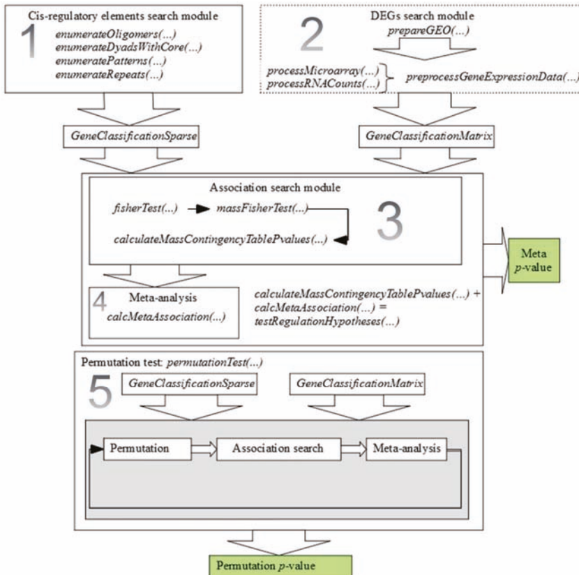
Figure 1. Scheme of metaRE modules that implement a five-step pipeline of the search for cis -elements significantly associated with differential gene expression over multiple datasets. DEGs—differentially expressed genes. Different modules are highlighted with squares; final sets of p -values are painted green. Described in the Methods steps are enumerated on the figure.
