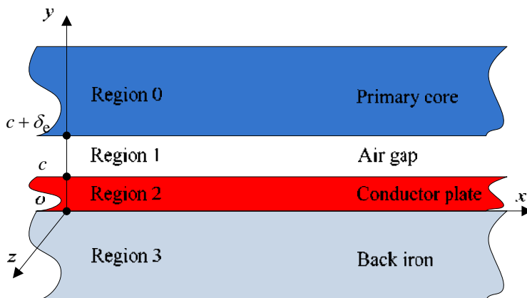
Figure 5. Two-dimensional multi-layer model.
