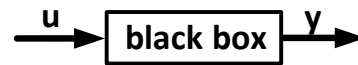
Figure 6. The black-box concept. We know little about the system, but we can learn from the input u - output y behavior.
