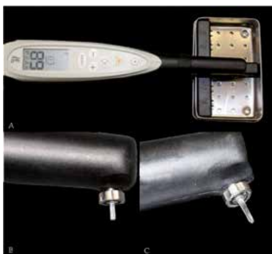
Fig. 6. (A) DIAGNOdent 2190 or DIAGNOdent pen calibration against the standard ceramic. (B) Occlusal tip. (C) Approximal tip.
