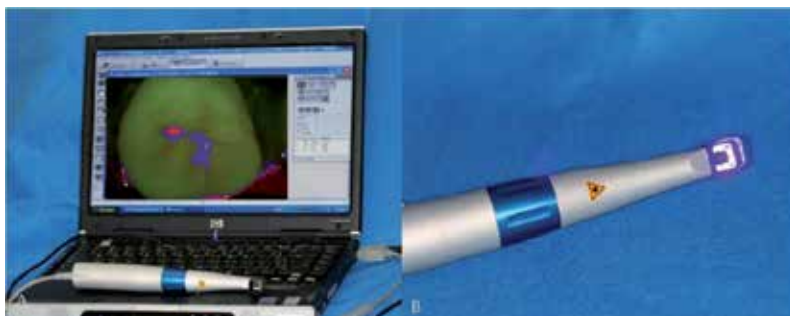
Fig. 8. (A) VistaProof fluorescence camera and DBSWIN software analysis. (B) Six blue LEDs emitting a 405-nm light.
