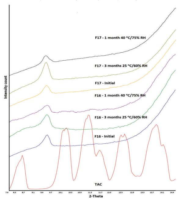
**Figure 9.** X-ray powder diffractogram of CAD and ASD formulations before and after storage at  $25 \,^{\circ}\text{C}/60\%$  RH and  $40 \,^{\circ}\text{C}/75\%$  RH conditions.
