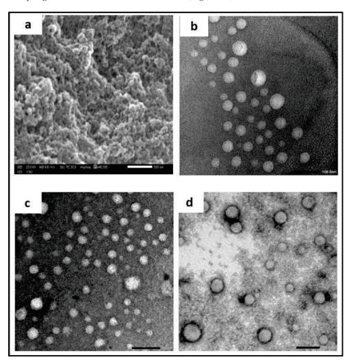
**Figure 3.** (a) SEM of NS with measurement of pore size. Magnification  $\times$  40 K, scale bar represents 500 nm. TEM images (b–d) showing the morphology of (b) NS, (c) FS-NS, and (d) LF-FS-NS. Magnification  $\times$  30 K, scale bar represents 100 nm.
