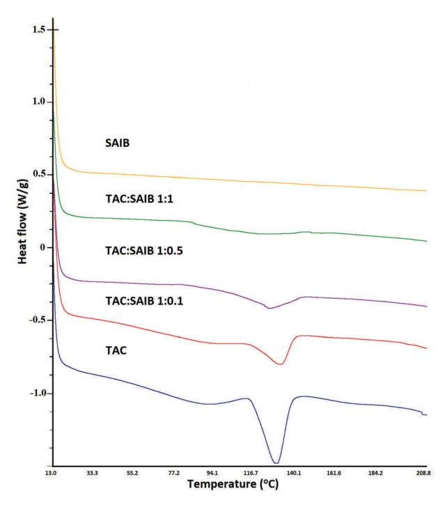
Figure 5. DSC thermograms of tacrolimus, SAIB, and various solutions / dispersions of drug and SAIB.
