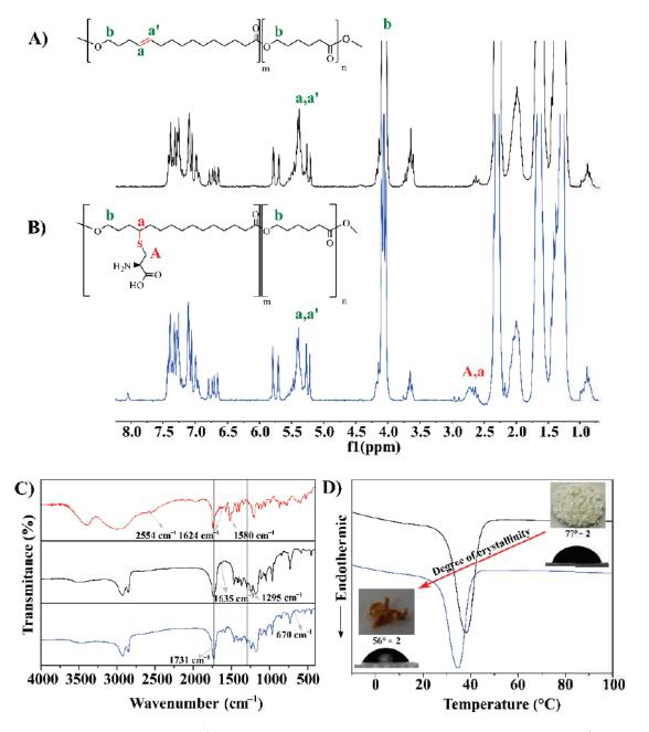
**Figure 1.** (**A**) <sup>1</sup>H NMR spectra of PGICL with peak assignments (a, a', b). (**B**) <sup>1</sup>H NMR spectra of PGICLCys (50/50 Gl/CL weight ratio) with peak assignments (a, a', b, a, A). (**C**) FTIR spectra of cysteine (red) and respective copolymers PGICL (black) and PGICLCys (blue). (**D**) Second run DSC heating curves of PGICL (black) and PGICLCys (blue) with different respective contact angle.
