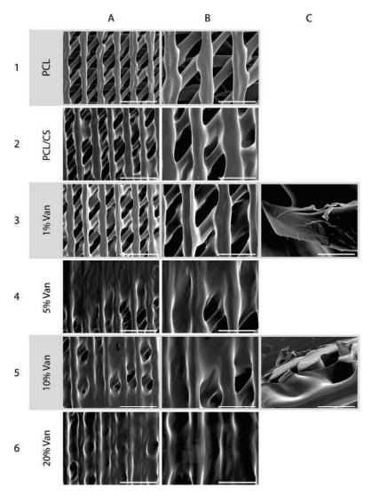
**Figure 5.** SEM micrographs of the (1) PCL, (2) PCL/CS, and (3–6) PCL/CS/Van scaffolds loaded with 1%, 5%, 10%, and 20% w/t vancomycin, respectively, at different magnifications: (A1–A6) 22×, scale bar 2 mm; (B1–B6)  $40\times$ , scale bar 1 mm; (C3) scale bar 200  $\mu$ m; (C5) scale bar 700  $\mu$ m.
