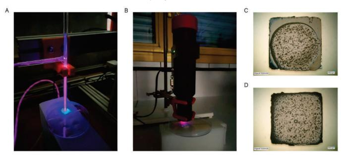
**Figure 3.** Plasma treatments performed on the PCL scaffolds. (**A**) Cold atmospheric plasma jet; (**B**) homemade torch with a piezoelectric plasma generator. Optical microscopy images of (**C**) Solid PCL scaffold (untreated) coated using CS hydrogel (scale bar 400  $\mu$ m); (**D**) solid PCL scaffold coated using CS hydrogel after being exposed to cold plasma for 30 s (scale bar 400  $\mu$ m).
