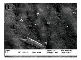
Figure 1. (A) TEM image of BCN; and (B) SEM images of the freeze-dried BCN.
