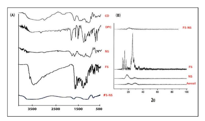
**Figure 5.** (A) FTIR spectra for FS-NS and its components; (B) X-ray diffraction pattern of FS, NS, and FS-NS.
