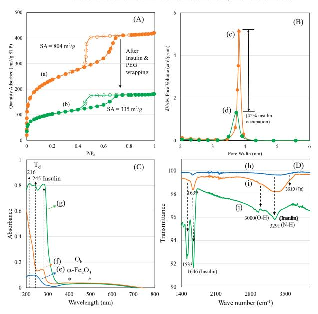
**Figure 2.** (A) Nitrogen adsorption isotherm: (a) ferrisilicate and (b) insulin/ferrisilicate/PEG. (B) Pore size distributions: (c) ferrisilicate and (d) insulin/ferrisilicate/PEG. (C) Diffuse reflectance spectra of (e) ferrisilicate, (f) insulin/ferrisilicate/PEG and (g) insulin. (D) FTIR spectra of (h) ferrisilicate, (i) insulin/ferrisilicate/PEG and (j) insulin.
