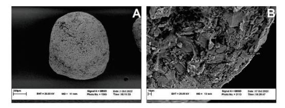
**Figure 6.** (**A**) Scanning electron microscopy of the coated BCNP and (**B**) the cross-sectional image of the coated BCNP.
