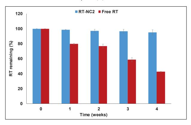
**Figure 1.** Percent remaining of RT as a function of exposure time to light for free RT and RT nanocrystals formulation RT-NC2.
