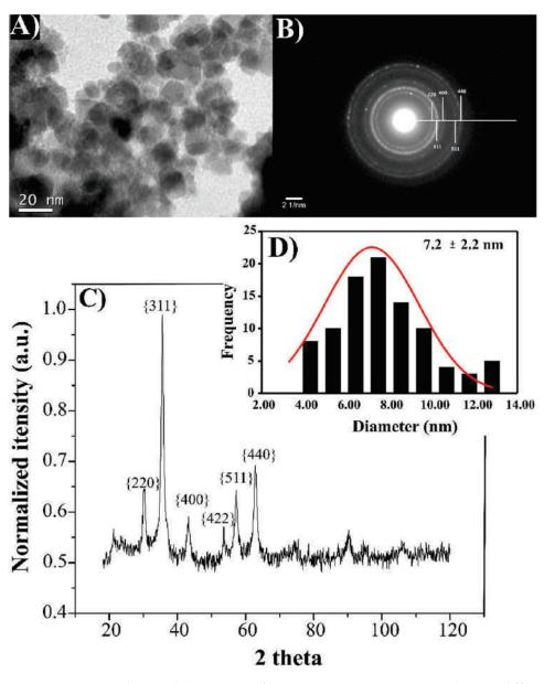
Figure 2. SPION@PGICLCys (A) Low magnification TEM image; (B) SAED; (C) XRPD diffractogram with diffraction peaks indexed to the spinel iron oxide phase. (D) Particle size distribution of the magnetic nanoparticles obtained from the TEM images.
