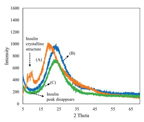
Figure 1. X-ray diffraction pattern of (A) insulin, (B) ferrisilicate and (C) insulin/ferrisilicate/PEG.
