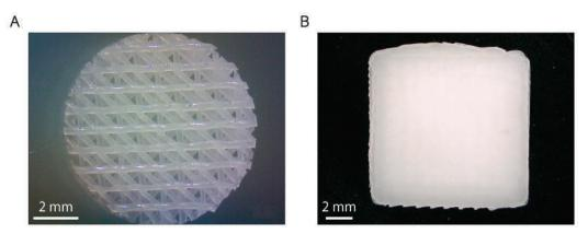
**Figure 2.** Micrographs of **(A)** porous and **(B)** solid PCL scaffolds printed using REGEMAT 3D Bio V1<sup>®</sup> bioprinter.
