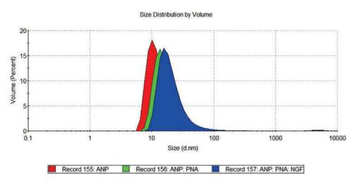
**Figure 1.** Nanoparticle characterisation through dynamic light scattering measurements. The hydrodynamic diameter increase of single- (ANP:PNA, green curve) and double- (ANP:PNA:NGF, blue curve) functionalised polyacrylamide nanoparticles resulted in a shift of size distribution compared to naked ANPs (red curve).
