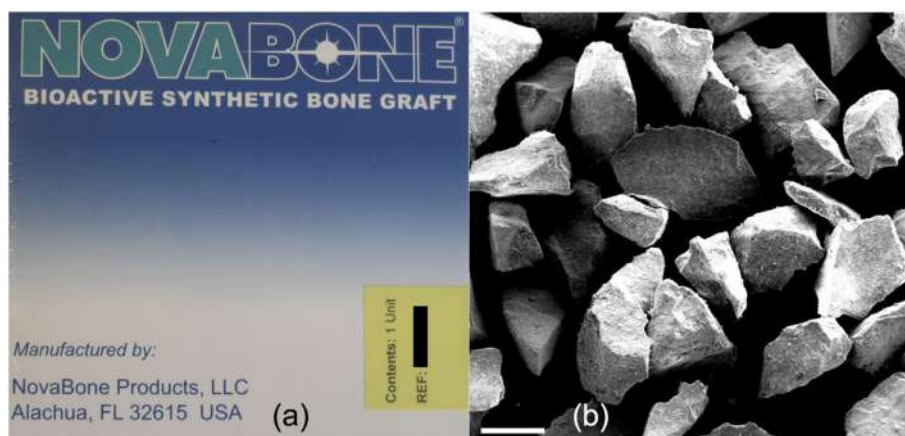
FIGURE 2 | (A) Packaging of NovaBone (45S5 Bioglass) powder for orthopedic applications and (B) scanning electron micrograph of NovaBone particles. Modified with permission from Jones (2013).
