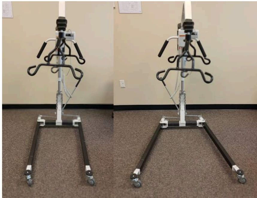
Figure 8.15 Portable Full-Body Mechanical Lift With Legs in a.) Closed Position and b.) Open Position
