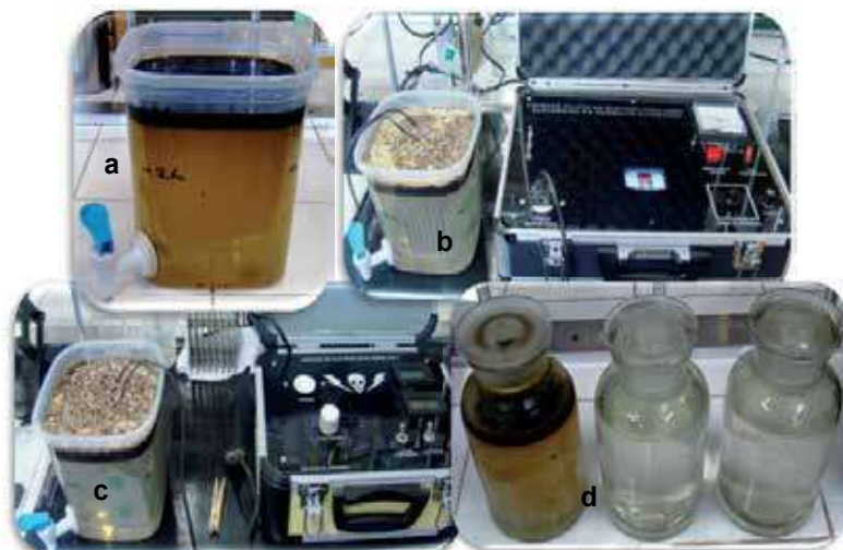
Figure 7. EF tests with real effluent with low salinity. Legend: a) raw effluent; b) effluent treated with AC electroflotation; c) effluent treated with DC electroflotation; and d) comparison of raw effluent with samples treated with AC and DC electroflotation. Note: The tests performed with t = 15 \text{ min} .
