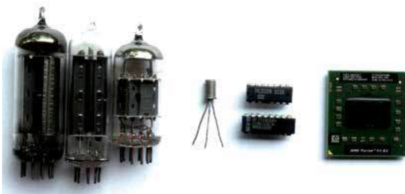
Figure 1. In order from left to right: three vacuum tubes, one transistor, two integrated circuits and one integrated microprocessor.
