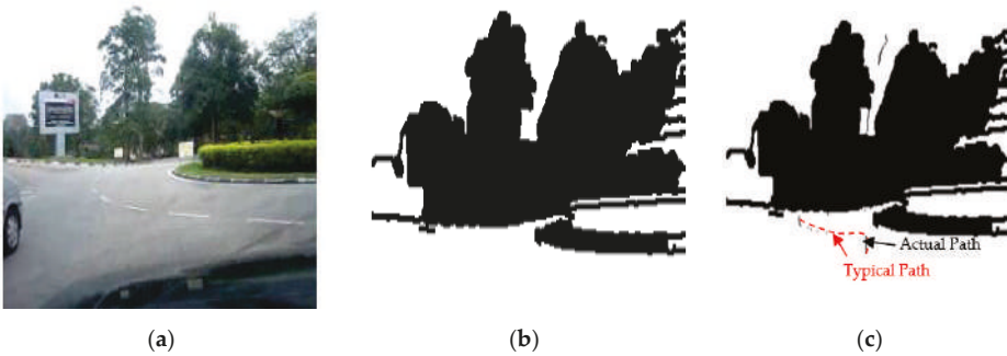
Figure 21. Autonomous detection and navigation of the proposed system in the road roundabout (with 5 m as diameter) with a car partially presented on the side/in front: (a) original image, (b) image processing, and (c) generation of the path within the road roundabout environment.
