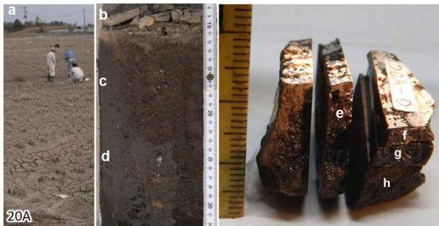
Fig. 6.18 An example sampling site for the radiocesium study. (a) Tsunami-affected farmland (sampling site No. 20A), (b) muddy tsunami deposit, (c) original soil 1, and (d) original soil 2 of this sampling site, (e) vertical section, (f, g, and h) horizontal sections (2–3 mm thick) of the muddy tsunami deposit (b)
