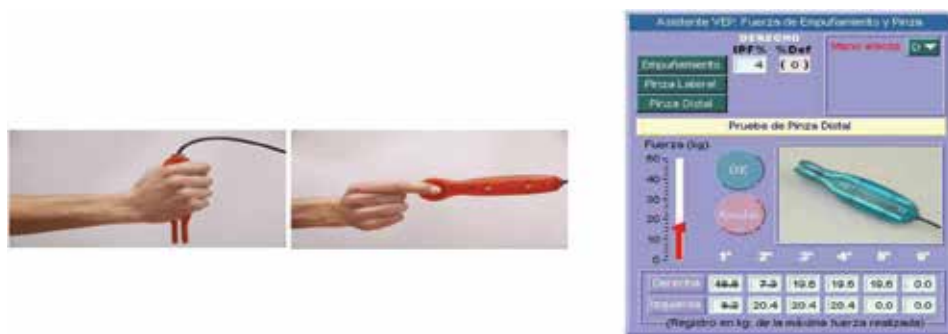
Figure 4. PC-based hand dynamometer used (probe detail).
