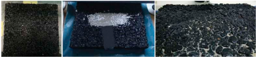
Figure 4. (a) Wet and clean surface (b) Contaminated surface (c) Contaminated surface after the rainfall simulation.
