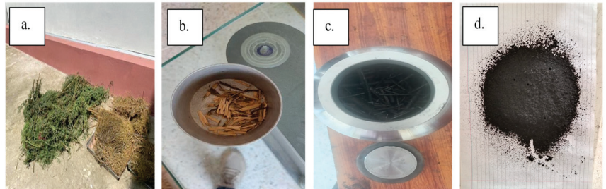
Figure 1. (a) Fresh Santa Maria feverfew plant, (b) dry plant, (c) biochar and (d) powdered biochar.
