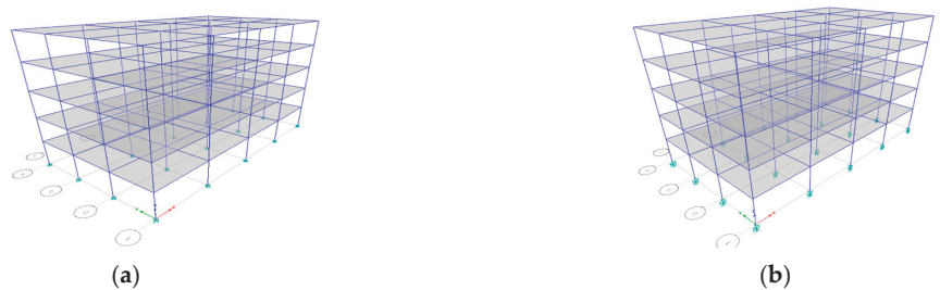
Figure 1. 3D View of the SMRF frame: (a) without base isolation; (b) with base isolation.
