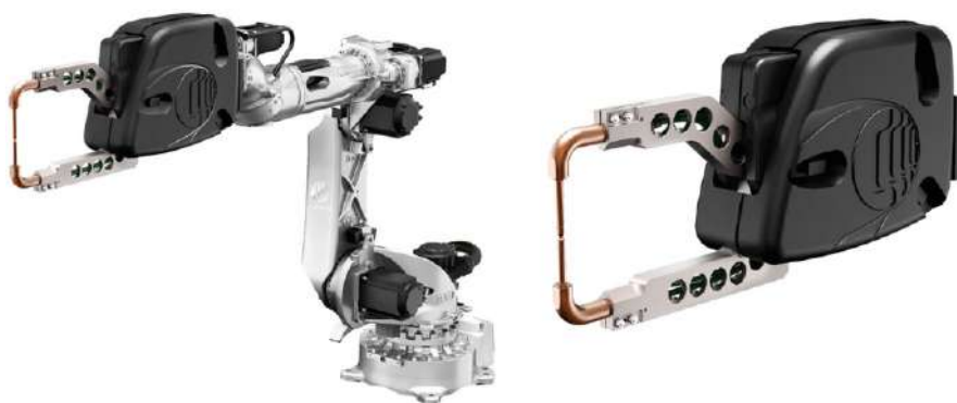
Fig. 7 Model of a COMAU robot and welding gun used for the welding of car parts
