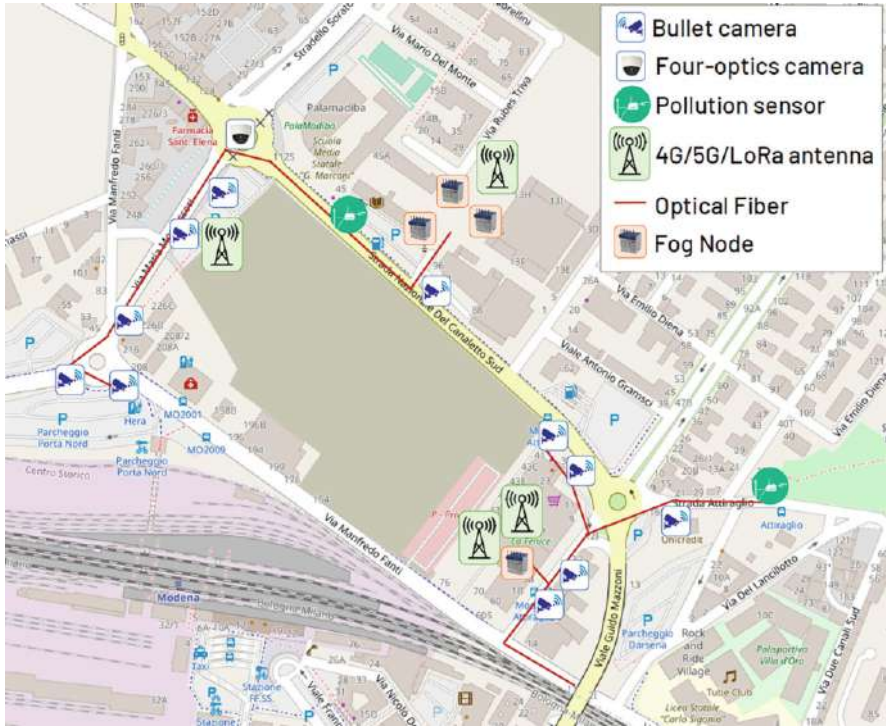
Fig. 7 Modena Automotive Smart Area (MASA) sensing, communication, and computation infrastructure
