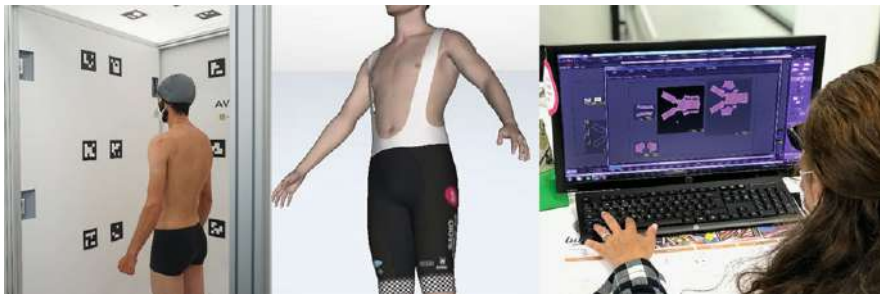
Fig. 14 Design process: scanner (left), 3D avatar (middle), pattern design (right)
