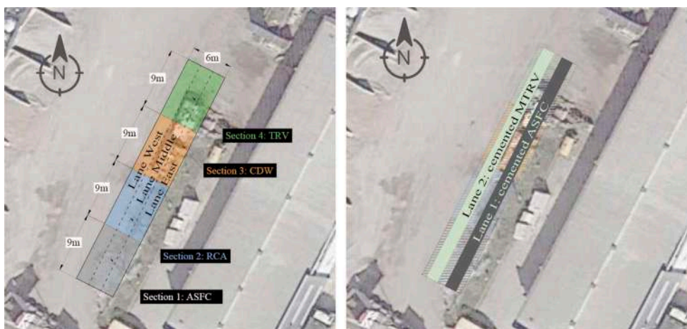
Figure 3. Schematic plan of constructed road and compaction lanes, Left: Sections of unbound materials and three lanes of roller compaction, Right: Cemented layers and lanes.
