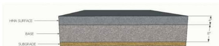
Figure 1. Pavement structure considered in the study.
