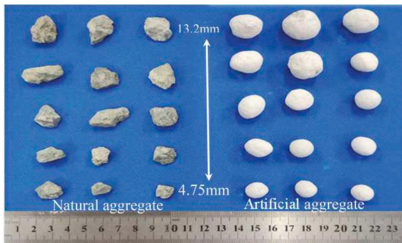
Figure 4. Images of natural aggregate and artificial aggregate with a size of 4.75-13.2 mm.
