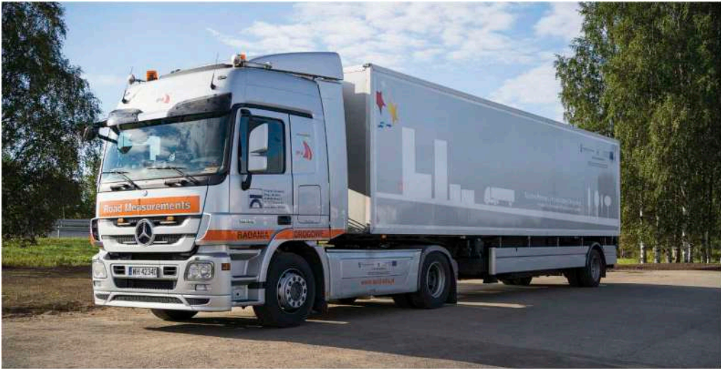
Figure 3. Traffic speed deflectometer truck, IBDIM Poland.
