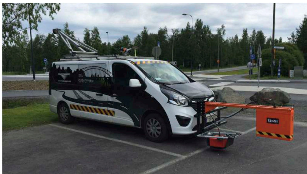
Figure 2. Roadscanners Road Doctor Survey Van. GPR antennas mounted in the front, lidar system, IMU, GPS and the cameras on the roof.
