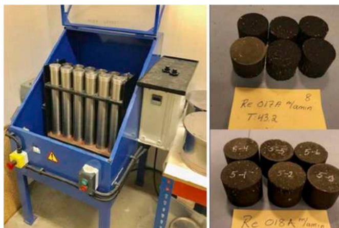
Figure 9. Apparatus and asphalt specimens for the vändskak-test (photo: O. Aslam).
