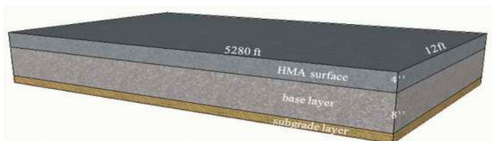
Figure 3. Pavement structure considered for the study.
