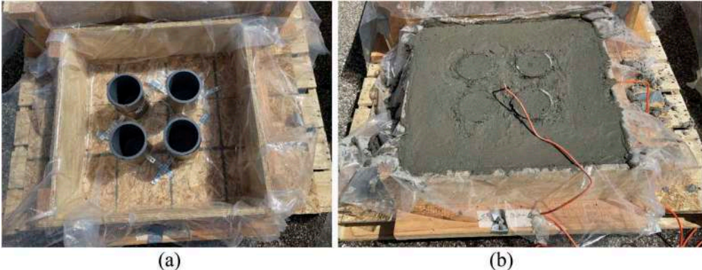
Figure 1. Photographic view of slab with four cast-in-place cylinders (a) before casting, and (b) after casting.
