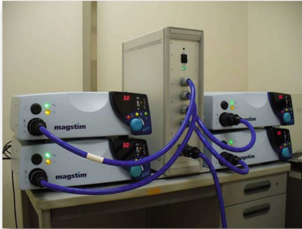
Fig. 2 Transcranial magnetic stimulator set up for QPS. Four monophasic magnetic stimulators are combined by a combine module
