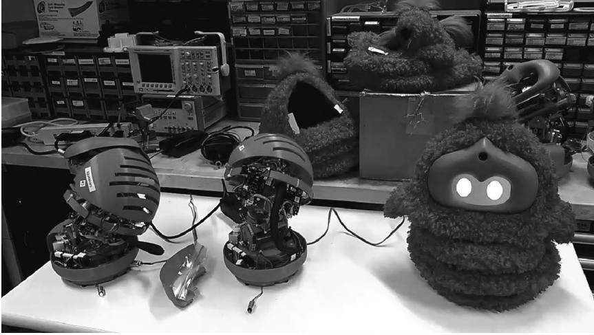
Figure 13.1c Tega robots, showing the electromechanical body on the left and covered in a fabric skin on the right. Personal Robots Group.
