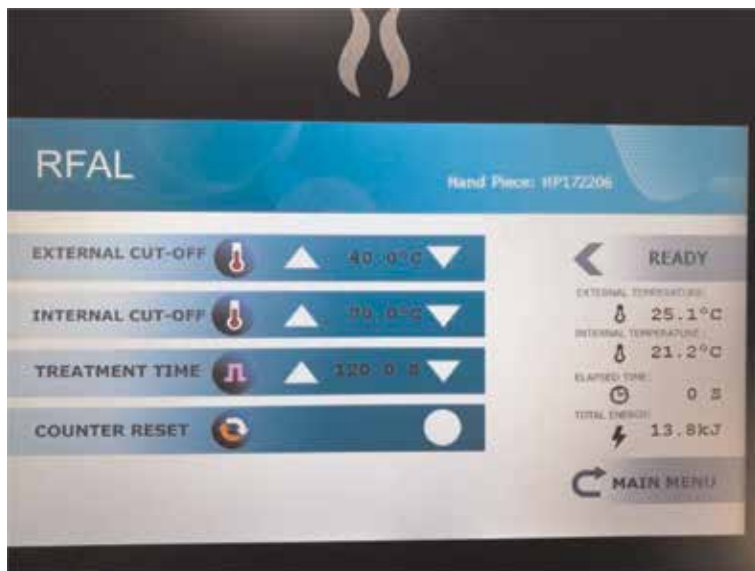
Figure 4. The GUI screen of the BodyTite® RFAL workstation. On the left hand side, the external (skin) electrode and internal electrode (adipose) cut off temperatures are set by the physician. Increments of 120 s of RF energy are dispensed and when the 120 s are up, double clicking on the foot pedal gives another 120 s. On the right-hand side are the real time temperatures of the external skin and internal fat temperatures as measured by the external electrode and internal electrode thermistors. As the user gets within 2°C of the cut off temperature, the audible beep that is emitted when RF energy is on, increases in tempo and when the cut off temperature is reached, either internal or external, the audible will sound that is characteristic for the external and one for the internal cut-off and the RF energy delivered is terminated to the hand piece and tissue heating stops. When the external and internal temperature is 0.1°C below the cut-off RF energy flow begins again. The automated feedback loop allows heating of the adipose and skin to occur together or independently and not exceed the pre-set amounts.
