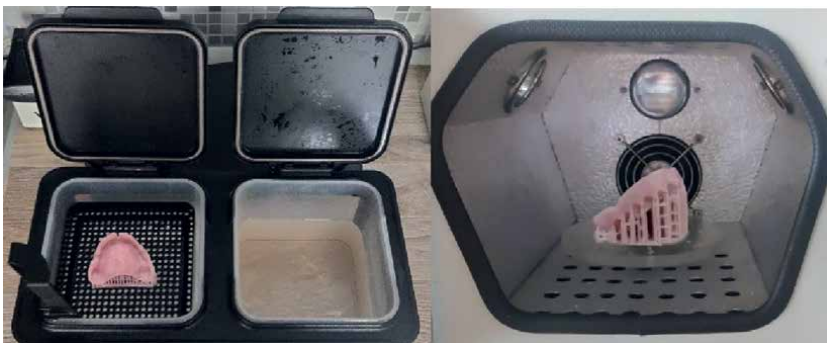
Figure 9. Post-processing of a SLA 3D printed denture base: Cleaning with isopropanol, and post-polymerization.
