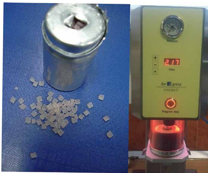
Figure 1. Thermoplastic polymer for injection, in a granular form; injection unit for thermoplastic resins.
