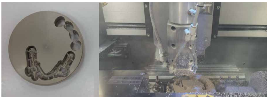
Figure 16. PEEK block for CAD/CAM milling; milling of a PEEK block.
