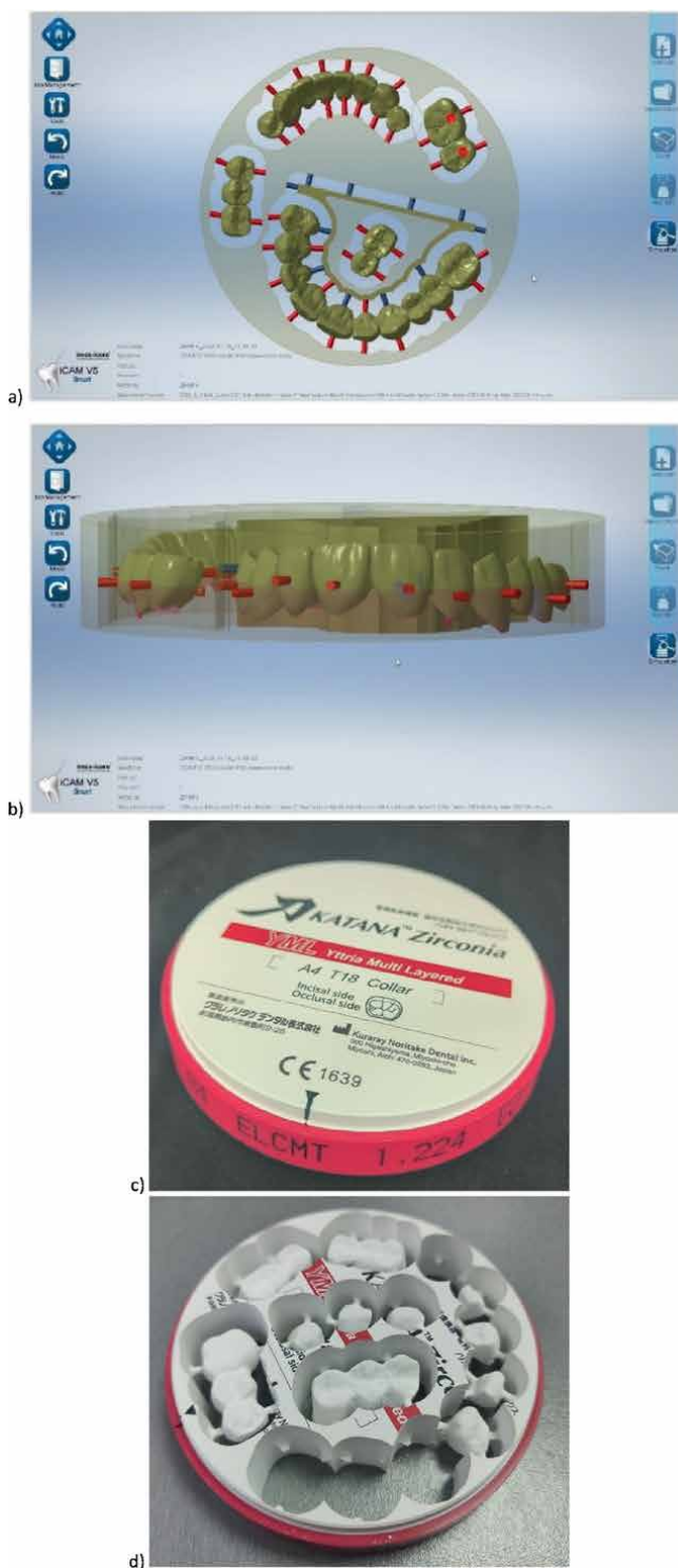
Figure 8. Photos a and b are print screens performed before starting the milling machine and pictures c and d are examples of a single block of material before and after it is milled.
